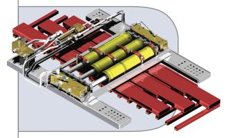
The large cylinder barrel size and the shorter cylinder length reduce deflection from the unloading forces.
