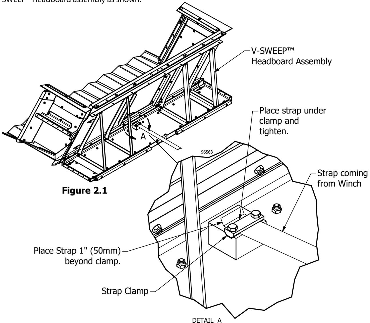
**Step 3: (Figure 3.1) Adjust wall guide:** Move headboard to the narrowest part of the trailer body, then Center and Square V-SWEEP™ headboard assembly. Adjust wall guides so there is 1/8" (3mm) clearance on both sides. Make sure that there are no welds, bolts, etc. that will be hit by the wall guides as the V-SWEEP™ headboard assembly moves from the front of the trailer to the rear.
