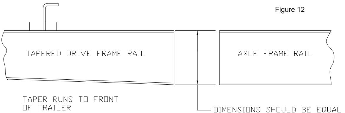
**NOTE:** Exact alignment of trailer centerline with the drive unit centerline is more important than alignment of the drive unit frame with the trailer's axle beams.
