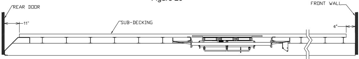
Figure 21 suggests a welding pattern. Starting each pass on the same side of the trailer gives sufficient cooling time.
