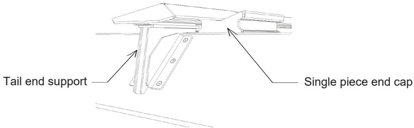
**Note 1:** Tail end supports need to be added after the floor slats are installed to ensure proper installation height.
