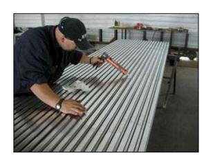
AFTER APPLICATION OF SIKAFLEX® PUSH SEAL AGAINST SLAT AT EACH AREA THAT SIKAFLEX® IS APPLIED.
