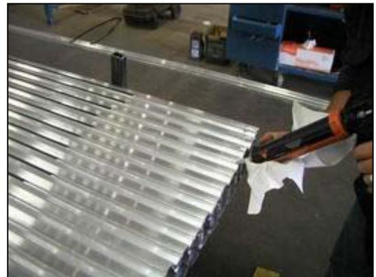
**NOTE:** The bead should be 2" long for the BLUE SEAL.
