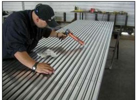
AFTER APPLICATION OF SIKAFLEX® PUSH SEAL AGAINST SLAT AT EACH AREA THAT SIKAFLEX® IS APPLIED.
