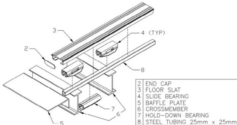
**NOTES:** The first three options include a wear pad bearing in the floor slats/planks. The square sub-deck material can extend to 12mm from the doors for all options.
