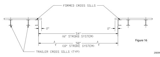
Weld or huck bolt the square tubes to the cross members between the jigs. Move the jigs and make a connection at each intersection of a tube and a crossmember. Welds should be 1/8" fillet, 3/4" to 1 1/4" long, and centered on the flange. Excessive welding and too little cooling will cause cross-members to warp.
