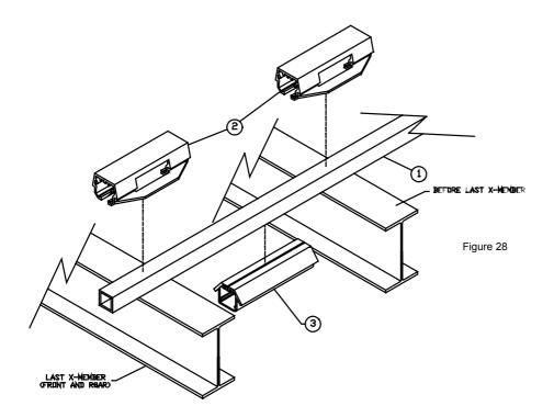
1 SUB-DECK SLIDE BEARING 3 HOLD-DOWN BEARING
