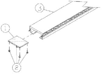
1 WEAR PAD BEARING 2 SCREW (4) 3 FLOOR SLAT
