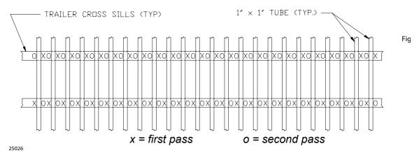
If aluminum profile is welded, put the two legs of the U down. If bolting, turn the tube over (Figures 18 and 19). Packing tape or paint should separate aluminum profiles from steel cross-members to prevent metal decay.
