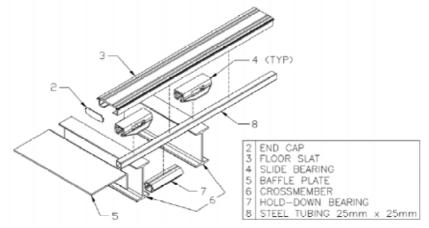
**NOTES:** The first three options include a wear pad bearing in the floor slats. The square sub-deck material can extend to 1/2" from the doors for all options.
