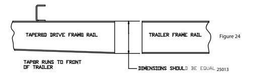
**NOTE:** Exact alignment of  $1^{\circ} \times 1^{\circ}$  tubing with the drive shoes is more important than alignment of the drive unit frame with the trailer's axle beams.
