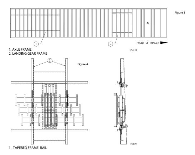
**NOTE:** Manufacturers of frameless trailers may want to consider extending their axle rails far enough forward that a frameless drive unit can be installed (extend 113" for 10" stroke, 109" for 6" stroke).
