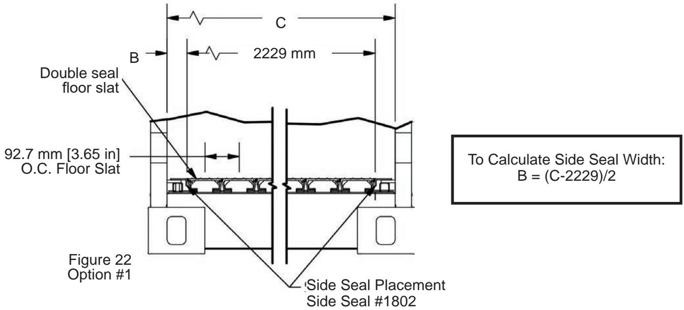
**Option #1:** Side Seal #1802 requires 32 mm [1-1/4 in] shim and one double seal slat.
