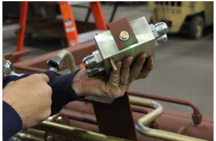
•The Control Valve can now be removed. Repeat steps in reverse order to replace the Control Valve.
