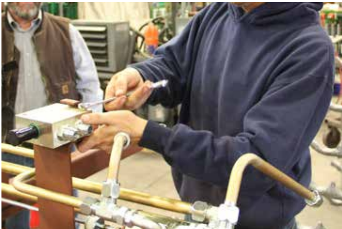
•Position a 9/16" wrench on the head of one of the bolts securing the Control Valve body to the drive frame bracket.
