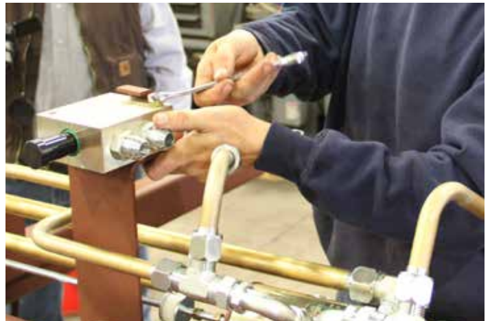
•Position another 9/16" wrench on the bottom of the bolt, removing the nut and lock washer. This will free the bolt.
