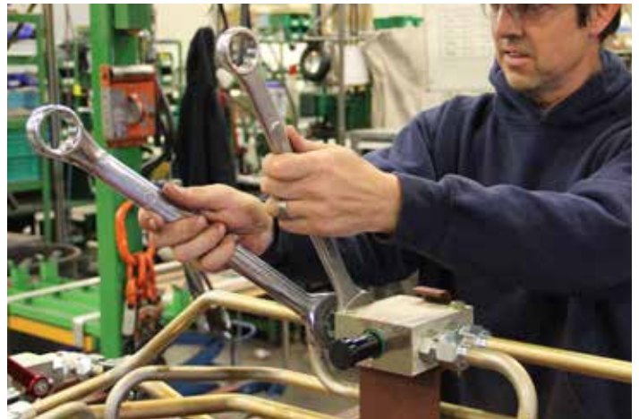
•At Control Valve end, loosen fitting using 1-1/8" wrench and a 1-1/4" wrench.
